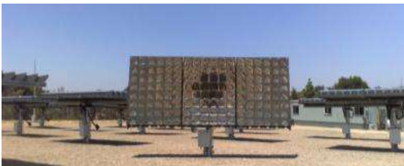
Fig. 28. View of an array so that the photographer is within the angular field of the core modules. The remaining modules are in operation. In the back, maintenance and measures booth.
